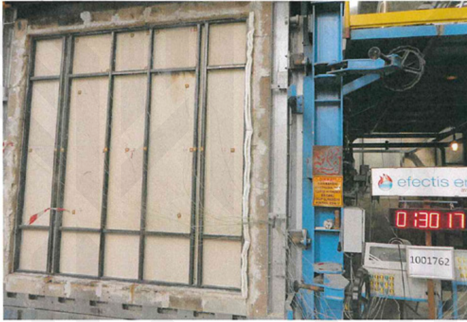
Photo C3: Unexposed side of the test specimen at 90 th minute of the test
