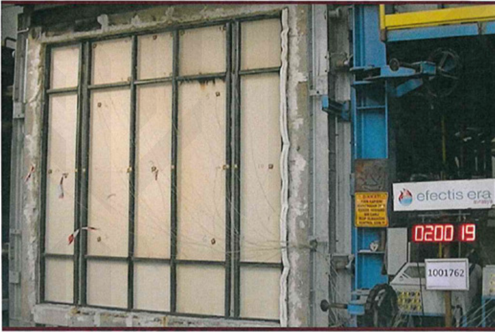
Photo C4: Unexposed side of the test specimen after the test
